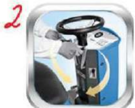
Turn on water & lower the brush head & the squeegee
